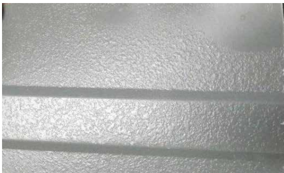
Storage corrosion under the paint on formed, nested panels.
