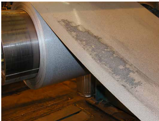
Heavy oxidation between coil wraps.
