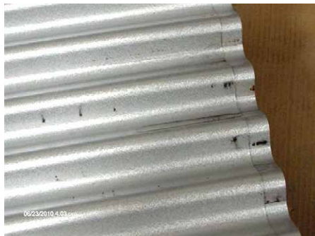
Transit abrasion on formed panels.
