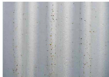
Moderate swarf staining on ZINCALUME Plus.
