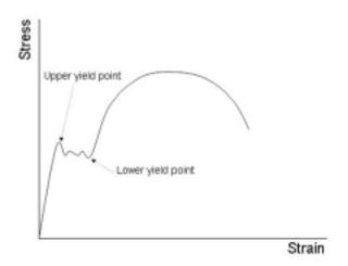
Product that does not exhibit these lines when formed is usually called non-fluting and is likely related to tension-leveling and/or temper passing practices after annealing.
