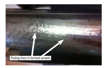
Fluting is a naturally occurring characteristic of annealed low-carbon steel and is influenced by the steel chemistry, cold-reduction practices and annealing cycles. It is associated with material that has an upper and lower yield point, or yield point elongation (YPE) and may also be referred to as Luder Lines, stretcher strain, or discontinuous/non-uniform yielding.
